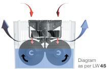
The basic idea behind the Venta Airwasher is brilliant in its simplicity: water is the filter. Air is drawn in and washed by the water.
