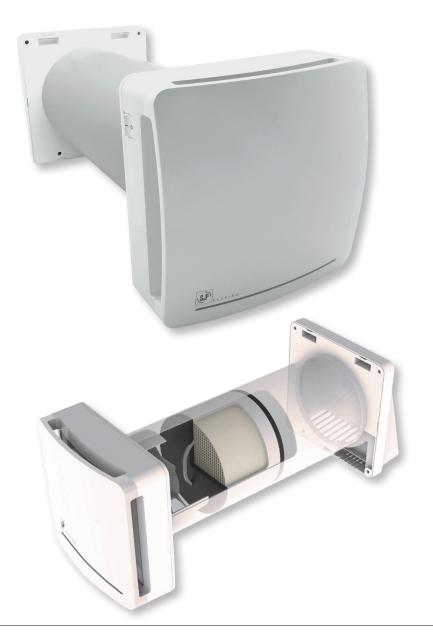
Decentralized ventilation unit, with heat recovery, for single rooms in domestic or commercial applications. Elegant design that allows its adaptation to any environment. Brushless motor with low comsumption electronic control. Ventilation system through an reversing motor and a heat exchanger with a performance up to 93%. Designed for a continuous operation, the unit adjusts the airflow proportionally to the humidity level (model RD), ensuring excellent indoor air quality.
