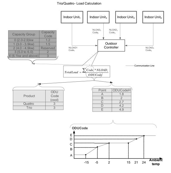
Compressor speed will be set between the minimum speed and the max speed according to the ODU NLOAD
